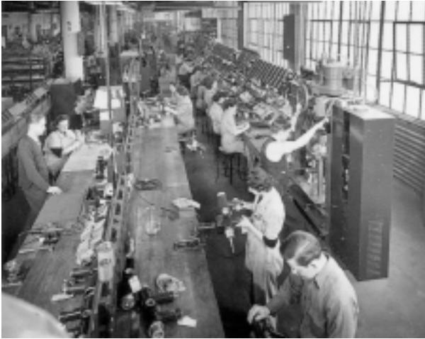
13 Factory production of X-ray tubes used on the US Army X-Ray Field Unit, 1942 – 1943
