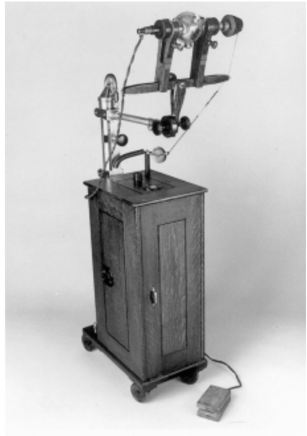
6 Mobile X-ray unit, designed by Dr Harry Waite and used by expeditionary forces in Europe during World War I circa 1916 – 1918. Notice exposed high voltage wires.
