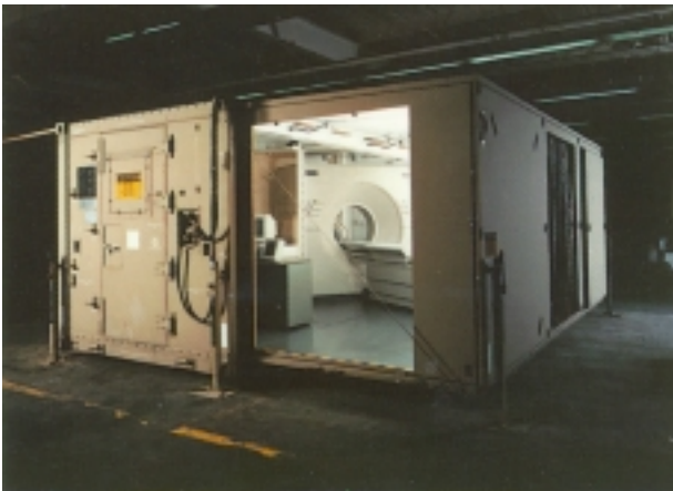
22 Picker IQ Premier CT Scanner, installed in a military ISO shelter. The unit shown saw service in Saudi Arabia in 1991 (Operation 'Desert Storm') and Somalia.
