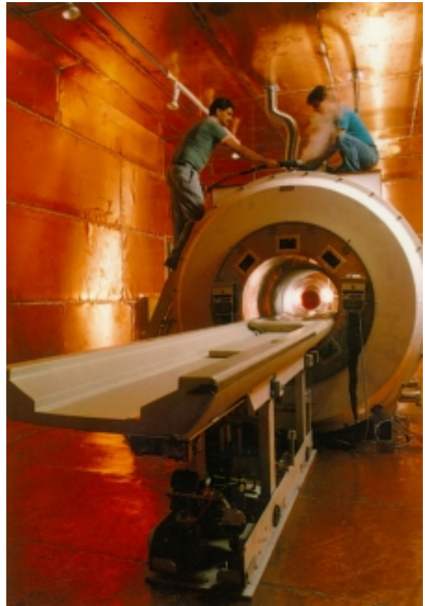
24 A Vista™ Magnetic Resonance Unit undergoing final assembly
