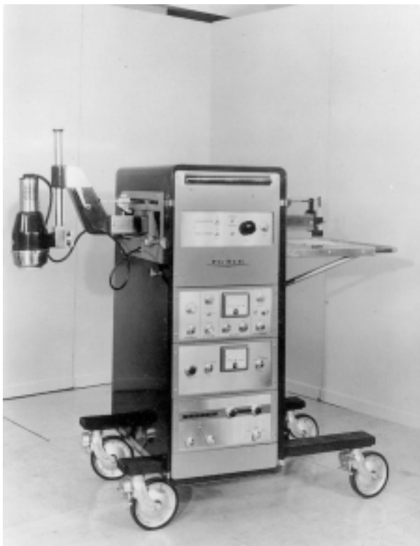
25 Picker Magnascanner (1958) vacuum tube model, later replaced with a transistorized model
