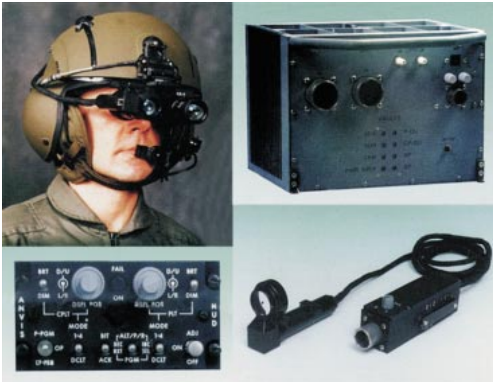
11 AN/AVS-7 NVG HUD fitted to a flying helmet
